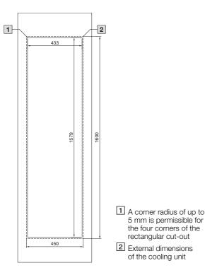
Mounting cut-out SK 3186.930, SK 3187.930, SK 3188.940, SK 3189.940 for 500 mm deep enclosures (external mounting only)
